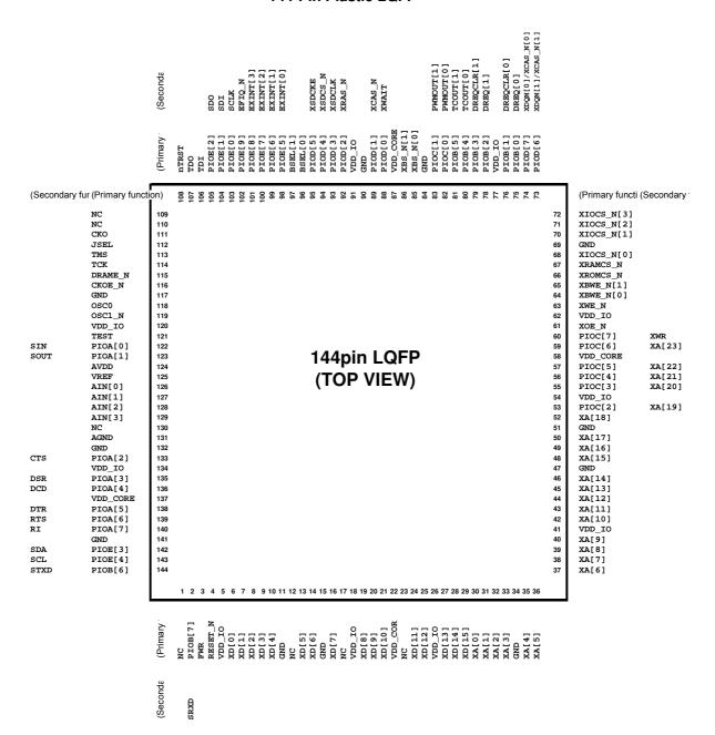
Notes: NC pins are electrically unconnected in the package. NC pins can be connected to Vdd or GND.
