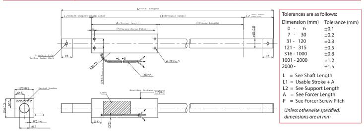
Note: Cable length 300mm. The bending radius of the motor cable should be 10.72 mm (wire diameter 1.34 \* 8) as suggested by the wire manufacturer. This radius should be maintained. Use supplied connector to attach the proper high-flex cable as required by your application.
