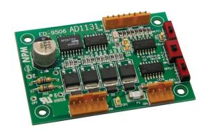
Nippon Pulse's AD1131 is a constant voltage driver board designed for 2-phase unipolar stepper motors.
