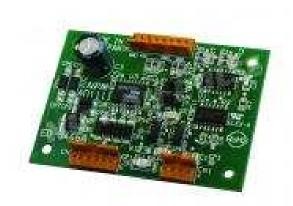
Nippon Pulse's AD1111 is a constant voltage driver board designed for 2-phase unipolar stepper motors.
