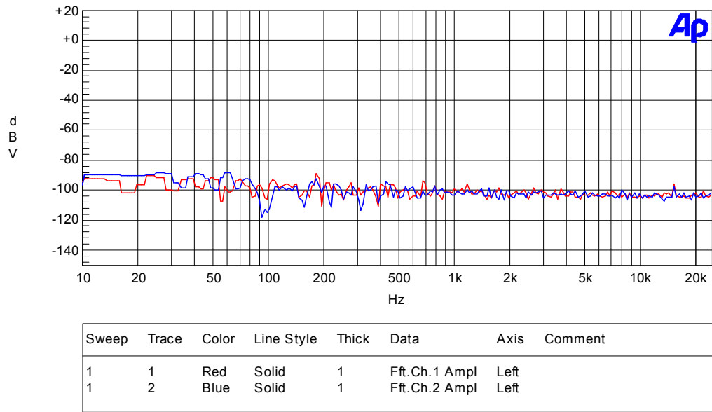
No signal, Self Oscillator @ 400kHz Fig 6, IRAUDAMP6 Noise Floor
