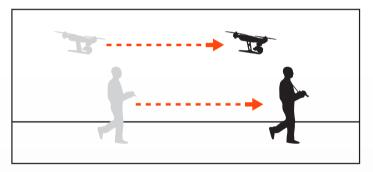
**Important Note:** In Follow Me function, the aircraft will maintain a constant altitude and cannot detect obstacles. Pilots who change their altitude by for example, moving to higher ground, during flight should be mindful of this.
