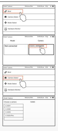
Step 6) Tap the 'Bind' button and select the 'CGO3\_XXXXXX' camera listed in the column under 'Camera', then enter the password '1234567890' when prompted and tap 'OK' after the connection has been established.
