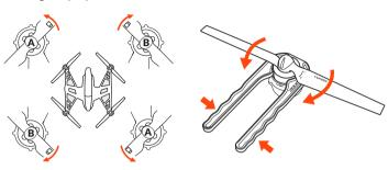
Each motor and propeller are marked with an 'A' or 'B' to ensure easy installation in the correct positions (for example: install propellers marked with 'A' on motors marked with 'A').
