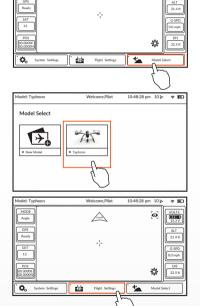
**Step 2)** Tap the 'Model Select' button, and if required press 'OK' to bypass any pop up warnings/alerts.
