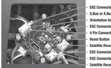
ESC Connector S.Bus or X.Bus Connector Orientation Arrow ESC Connector 4 Pin Connector (factory use only) Reset Button Satellite Receiver Connector ESC Connector ESC Connector
