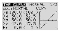
Make sure that your throttle curve is linear. The motor's transition time from forward to reverse can be reduced by setting points a few % above and below midstick, making the throttle curve as steep as possible between those points. Before testing your setup, remove the props from the motors. Turn on the transmitter and connect the battery to the Voltage 500 3D. Use the LED codes on the Flight Controller to verify that Gear switch can select the Motor Disarm mode and the two flight modes.
