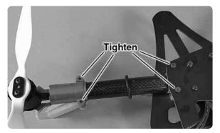
The Voltage 500 3D does not need any assembly. All the non-adjustable bolts have been set to the proper torque and have thread locking compound applied to keep them secure. The tension of bolts that clamp the booms should be checked before each flight by twisting each motor mount. If the boom is not tight, these bolts should be tightened.
