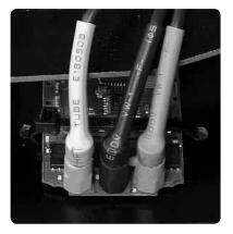
On the front left and rear right ESC, the colors on two of the wires will not match the sockets.
