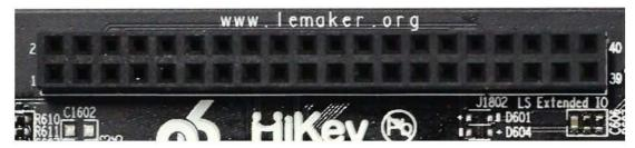
The low speed expansion connector carries GPIO and other low speed interfaces. The connector is a low profile 40 pin female 2mm receptacle (20x2) of a specified height of 4.5mm height.
