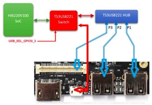
The HiKey board utilizes a single SoC USB interface without USB protocol hardware split utransfer support. The USB interfaces are therefore subject to the following restrictions:
