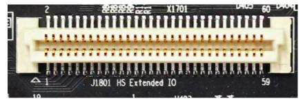
The following table shows the High Speed Expansion Connector pin out:
