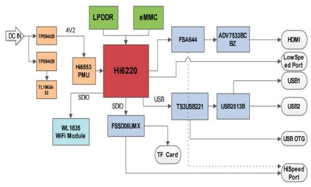
The 96Boards specification defines how power arrives to the board and few supplies that the board needs to provide. The on board power requirement for each 96Boards implementation depends on the SoC and the set of peripherals that are specific to that implementation.
