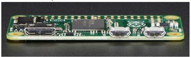
The most intriguing difference for hackers and makers is that the Pi Zero does not come with the soldered GPIO header. Partially this is to save cost, but it also allows the Pi Zero to be very thin and gives you the option of embedding it easily into a project box.
