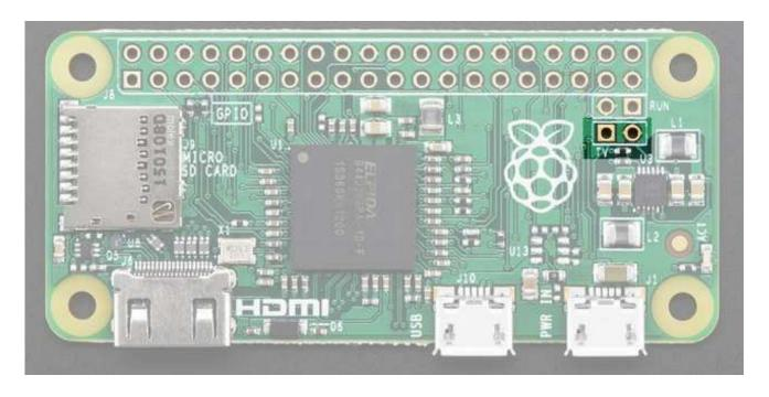
The hole on the left, nearest to the **TV** text, is the signal (+) line, the pin to the right of it is the ground (-) line. Solder two wires to these pads and connect them to an RCA Jack (http://adafru.it/2792) like this one
