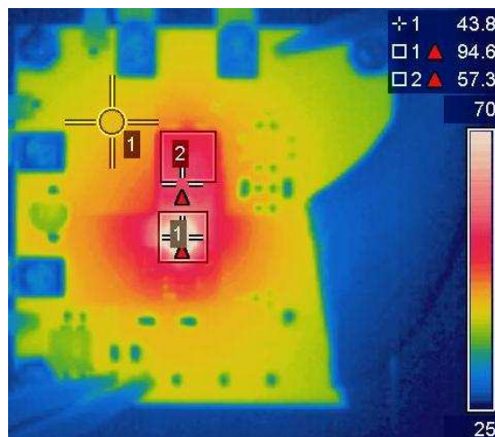
Figure 21: Thermal Image at V_{IN} = 12V , I_{OUT} = 10A (IR3475: 95^\circ C , Inductor: 57^\circ C , PCB: 44^\circ C )
