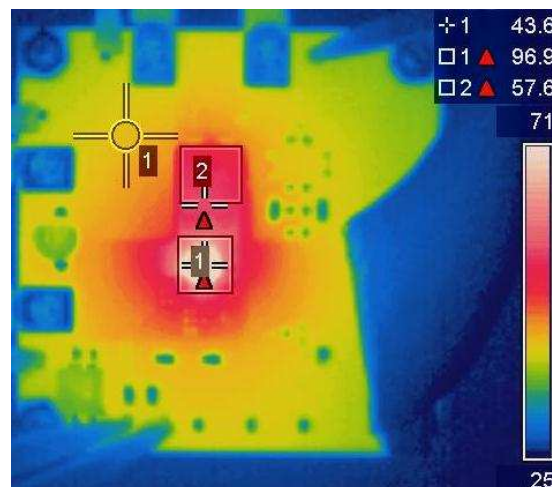
Figure 22: Thermal Image at V_{IN} = 19V , I_{OUT} = 10A (IR3475: 97^\circ C , Inductor: 58^\circ C , PCB: 44^\circ C )
