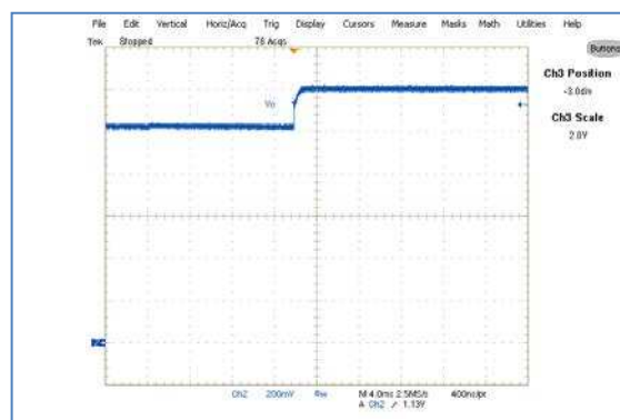
Figure 34: Start up with 1V pre bias 0A Load Ch2:V o
