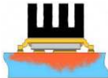
⑦ Mounted to a PCB with a thin gap filler and heat sink. (still air)
