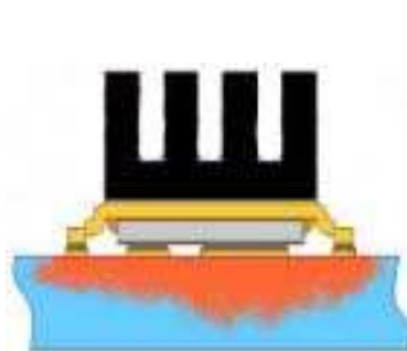
⑥ Mounted on minimum footprint full size board with metalized back and with small clip heatsink. (still air)
