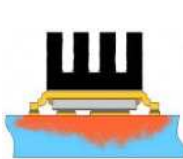
⑧ Mounted on minimum footprint full size board with metalized back and with small clip heatsink. (still air)
