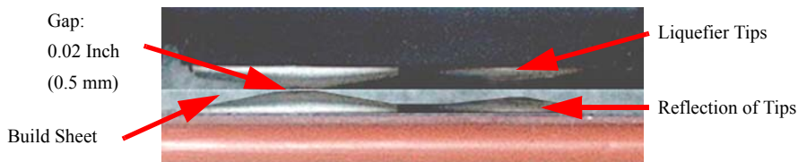
Figure 6-3: Manual Z Zero Calibration
