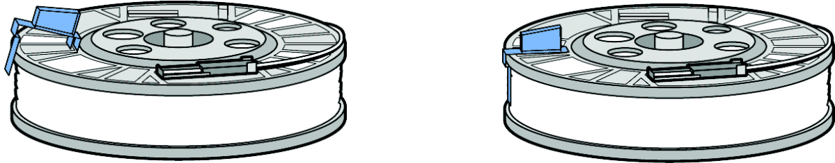
Figure 25 Installing material retaining clips
