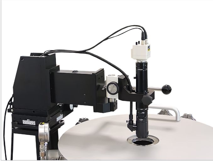
Optional high-resolution XY microscope movement (Left: working position. Right: tilted into parking position).
