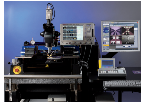
Automated multiport on-wafer measurements with the PA200 and VNA.
