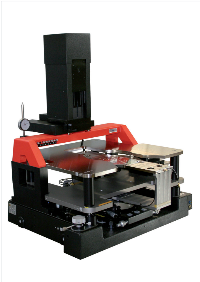
Setup prepared to integrate an OEM emission microscope camera system onto the microscope bridge.
