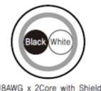
18AWG x 2Core with Shield
