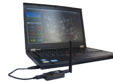
Ground station laptop with radio connected
