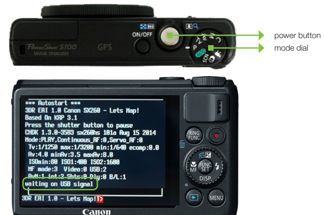
Camera ready to map: waiting on USB signal
