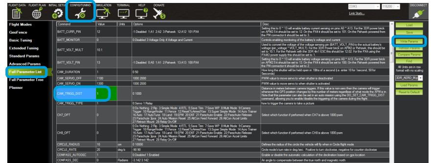
Mission Planner Full Parameter List: Set CAM_TRIGG_DIST to 1.
