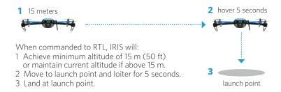
**Reposition during landing**: During landing, use the right stick on the controller to adjust IRIS' position.
