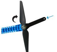
**To remove**, hold the motor in place with the propeller tool, and spin the propeller in the direction of the unlocking symbol.
