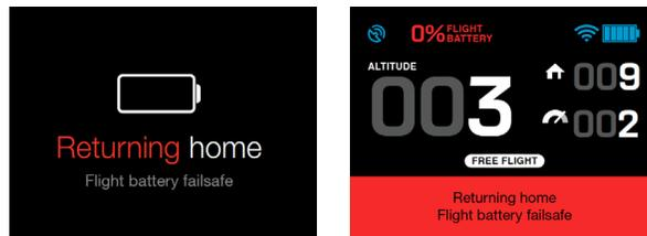
Figure 6.2.5.2: Controller - Critical Battery Alert
