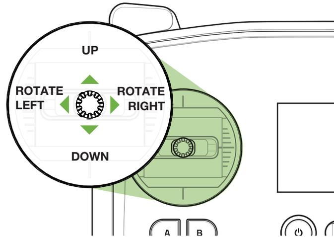
Figure 4.6.2.1: Controller Left Joystick
