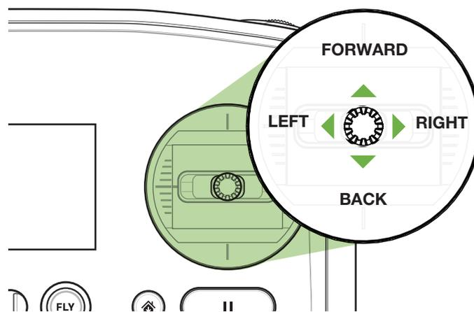
Figure 4.6.2.4: Controller Right Joystick Controls
