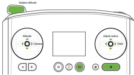
Figure 5.3.2.2: Orbit Controls
