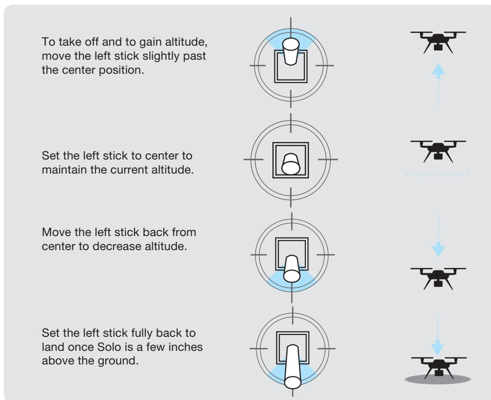
Figure 4.6.2.2: Throttle Joystick Behaviors
