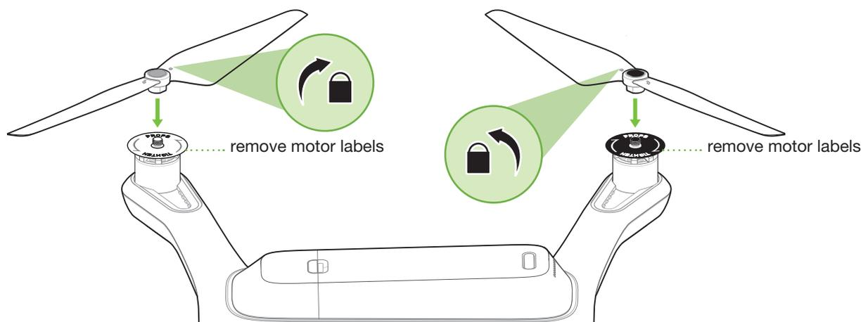
Figure 2.4.1.1: Attach Propellers
