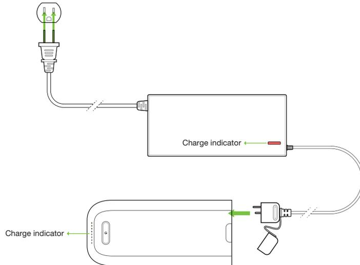
Figure 2.2.1.1: Solo Battery Charging
