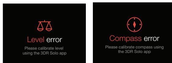
Figure 6.1.1.3: Controller - Re-Calibration Required Alerts
