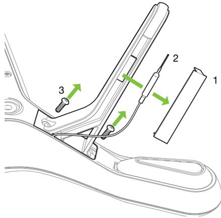
Figure 9.4.2.1: Detaching the Antenna from the Leg
