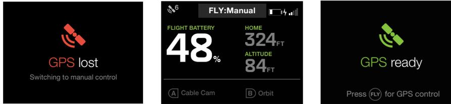
Figure 6.2.4.1: Controller - GPS Signal Alerts
