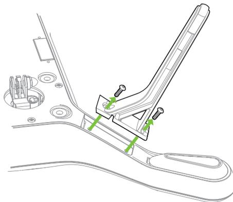
Figure 9.4.1.1: Standard Leg Replacement Process
