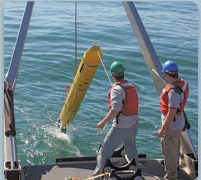
The Bluefin-12S can be recovered with a simple A-frame
