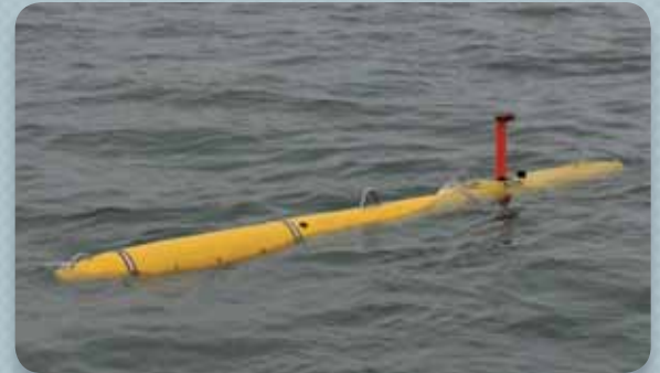
The Bluefin-12S operating as a sensor testbed
