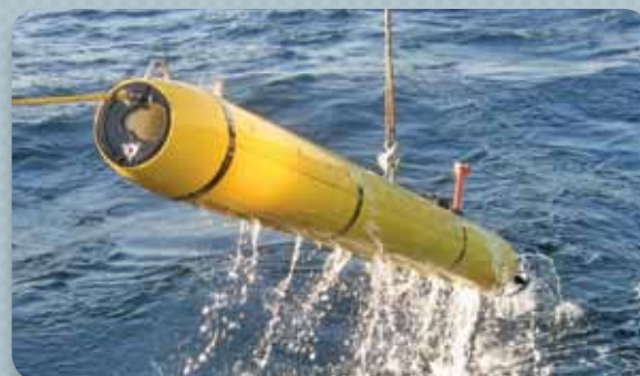
Pop-off nose releases a line for easier vehicle recovery
