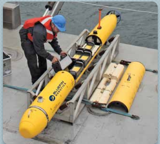
Swappable batteries facilitate rapid mission turnaround.
