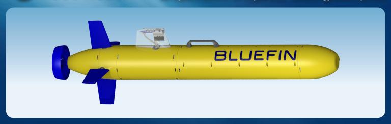
The Bluefin SandShark is a small, open-platform, autonomous underwater vehicle (AUV) designed for developers. SandShark combines a standardized low-cost tail with core vehicle systems, a large modular payload area, and an open development platform. This combination provides a flexible subsea "reference design" to support rapid technology development.
