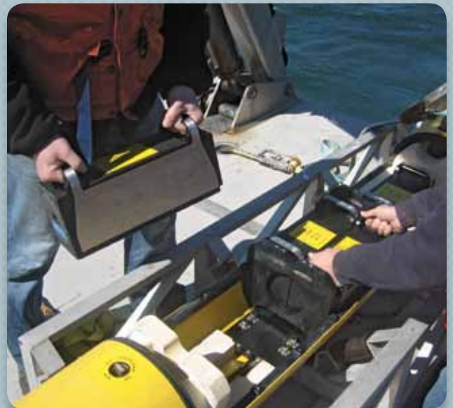
Batteries can be rapidly swapped in the field
