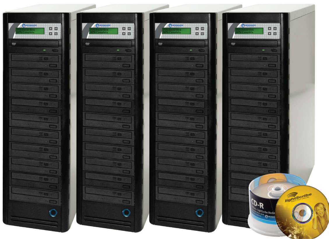
An example of four NET towers daisy-chained together to record 40 discs at once.
