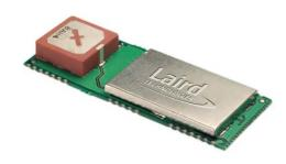
The Embedded Bluetooth® AT Module is designed for applications that demand a robust and reliable Bluetooth connection. This product is designed with solder connections for mounting directly onto a main PCB. The integrated highperformance, multilayer ceramic antenna is highly resistant to de-tuning, allowing great flexibility in positioning.
