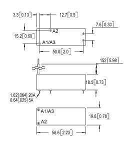
(1) PC pin versions carry 5 or 20 amps, see part number system. Flying lead and panel versions carry 30 amps.
