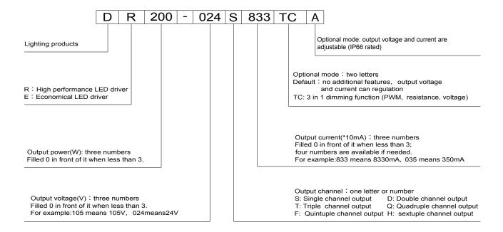
For example: DR200-024S833TC means it is a high performance LED driver, output power 200W, output voltage 24Vdc, output current 8330mA, single output, with 3 in 1 dimming function.
