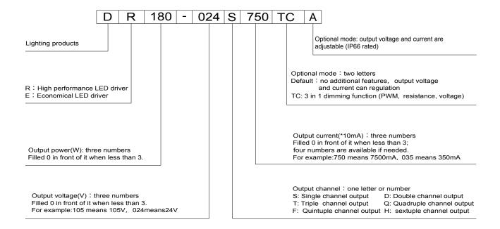
For example: DR180-024S750TC means it is a high performance LED driver, output power 180W, output voltage 24Vdc, output current 7500mA, single output, with 3 in 1 dimming function.
