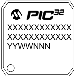
100-Lead TQFP (12x12x1 mm)
