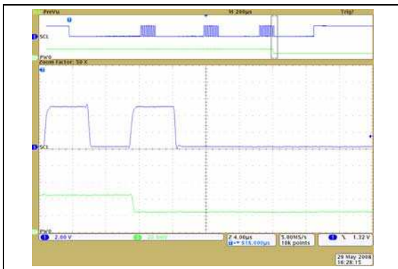
FIGURE 2-28: 10 k \Omega – Low-Voltage Decrement Wiper Settling Time ( V_{DD} = 2.7\text{V} ) (1 \mu\text{s}/\text{Div} ).
