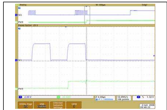
FIGURE 2-56: 100 k \Omega – Low-Voltage Increment Wiper Settling Time ( V_{DD} = 2.7\text{V} ) (1 \mu\text{s}/\text{Div} ).
