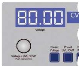
All these features contribute to an operator friendliness. With the LOCK push button the controls can be locked, in order to protect the equipment and the loads from unintentional misuse. An analog terminal on the rear of the unit provides functionality for parallel connection. Thus the devices can be combined into a complete system without much effort.
