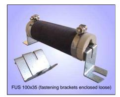
Cemented wirewound tubular fixed resistor, degree of protection IP00, with insertable fastening brackets which are enclosed loose, fixing parallel to mounting surface. Connections by screw, fast-on or soldering clips of the resistor\*.
