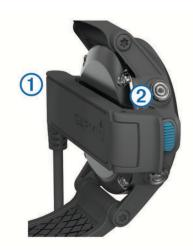
**4** Align the hinged side of the charger ② with the contacts on the back of the device.
