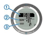
The race timer screen displays the race timer ①, time to burn ②, and distance to the start line ③.
