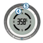
The two pointer marks 4 serve as a bearing pointer. The top blue mark 5 points in the direction you are facing.
