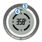
The two pointer marks @ serve as a bearing pointer. The top blue mark ⑤ points in the direction you are facing.
