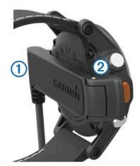
4 Align the hinged side of the charger ② with the contacts on the back of the device.
