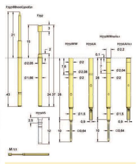
The F797 is the long travel version of the F772. These probes can be combined well in dual stage fixtures.
