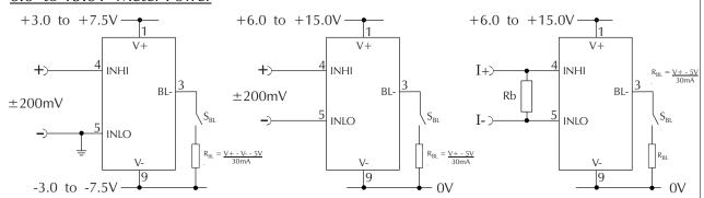
Measuring a single ended input voltage referenced to a split supply, i.e. the input voltage and the meter's power supply share the same 0V rail. Ensure solder link LCOM is open.
