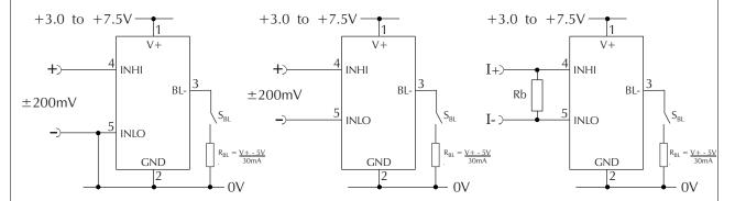
Measuring a single ended input voltage referenced to supply, i.e. the input voltage and the meter's power supply share the same 0V rail. Ensure solder link LCOM is open.
