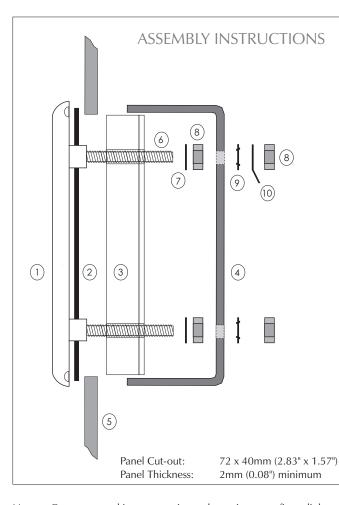
(1) Bezel Qty. 1 ② O-ring Qty. 1 Panel Instrument 4 Mounting Clamp Qty. 2 (5) Front Panel Screw Stud (6) Otv. 4 (7) **Insulating Washer** Qty. 4 Qty. 8 (8) Fixing Nut 9 Shakeproof Washer Qty. 4
