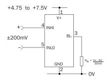
Measuring an input voltage referenced to a floating supply, i.e. the input voltage and the meter's power supply are isolated from each other. Ensure solder link LCOM is closed.
