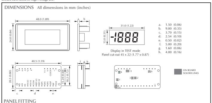
Fit the bezel to the front of the panel and then locate the meter into the bezel from behind. Alternatively the meter and bezel may be assembled
