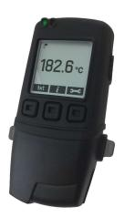
This standalone data logger measures and stores more than 250,000 temperature readings from a K, J or T-type thermocouple at a resolution of  $0.1^{\circ}$ C ( $0.2^{\circ}$ F). It comes supplied with a K-type thermocouple capable of measuring from -80 to +400°C (-112 to +752°F).
