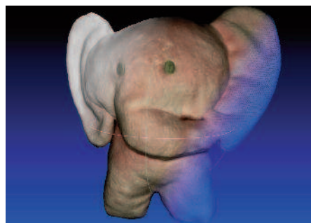
Hybrid 3D scan of a soft toy (color image, relief and wireframe)
