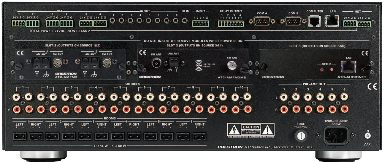
AES – Rear View with ATC-AMFM2, ATC-AMFMXMD, and ATC-AUDIONET Tuner Cards
