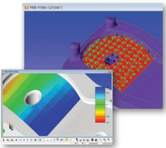
Surface deviation can be displayed as spherical points or as a gradient surface.
