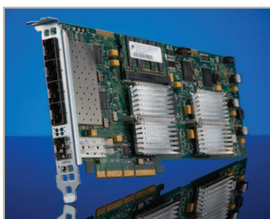
Figure 7. J6872A 10 Gigabit/Gigabit Ethernet high-performance interface card
