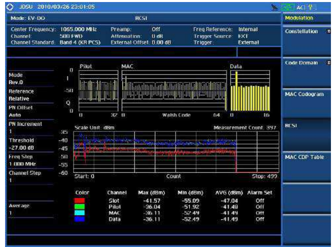
EV-DO received codestrength indicator
