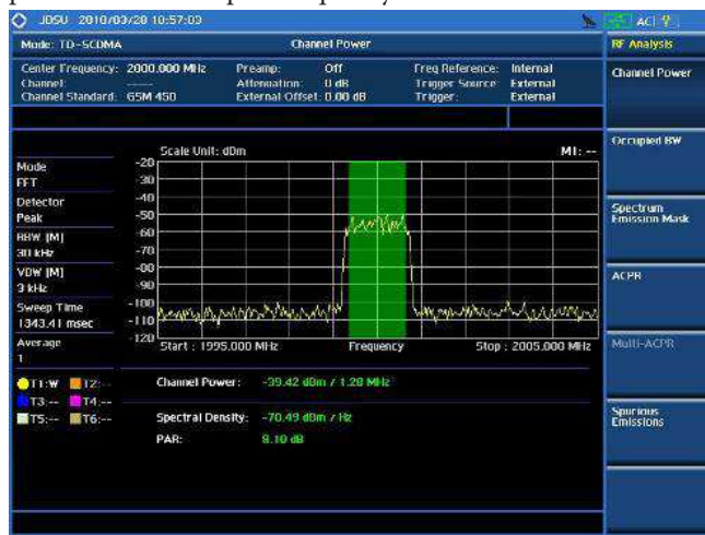
TD-SCDMA Occupied Bandwidth
