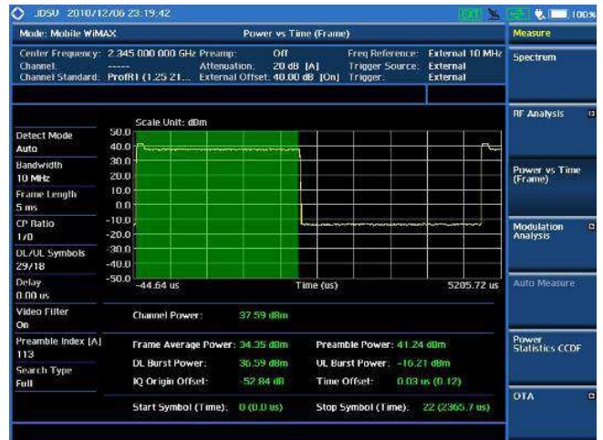
WiMAX Power vs. time (frame)
