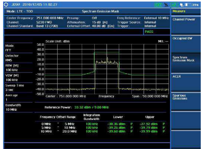
LTE spectrum emission mask
