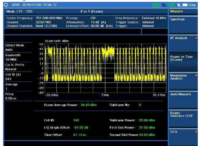
LTE Power vs. Time (Frame)
