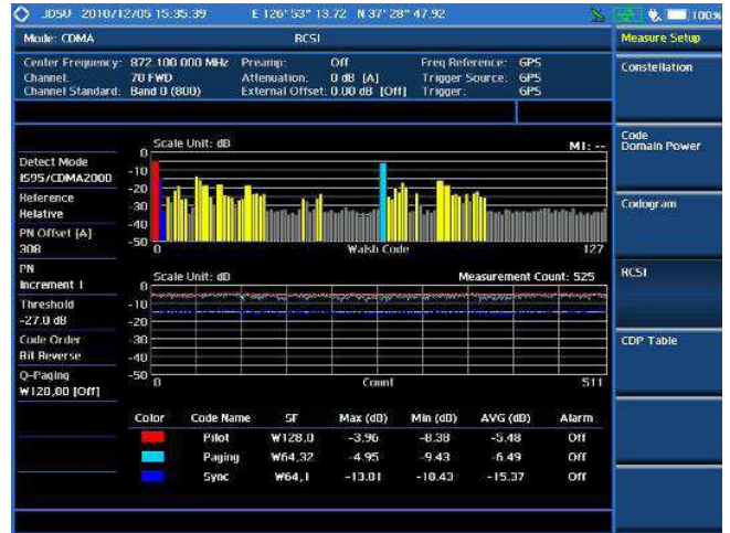
CDMA received code strength indicator
