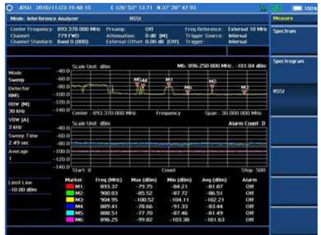
Received signal strength indicator
