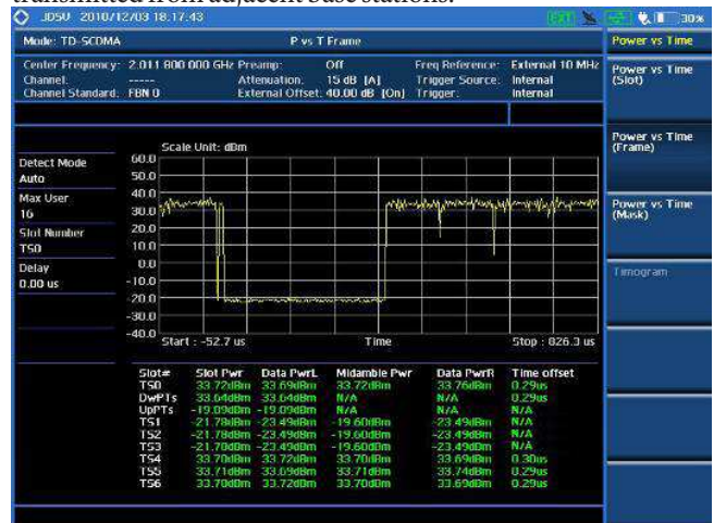
TD-SCDMA power vs. time (frame)
