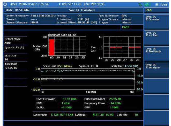
TD-SCDMA OTA sync-DL ID analyzer
