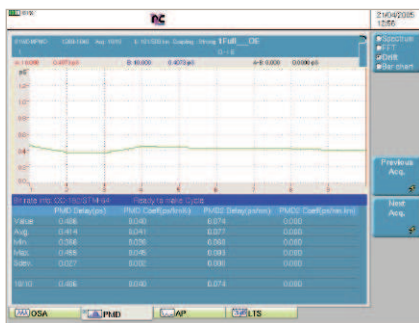
Long-term analysis with drift curve display
